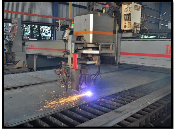
Batam Plant Equipment – NC Plasma Cutting Machine
