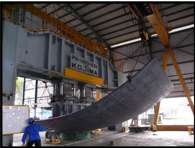
Batam Plant Equipment – 1,600 ton Press Machine
