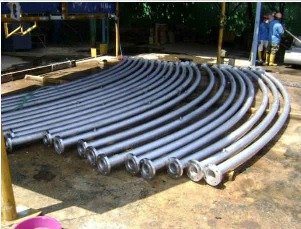
Water Spray Pipe [Carbon steel]
