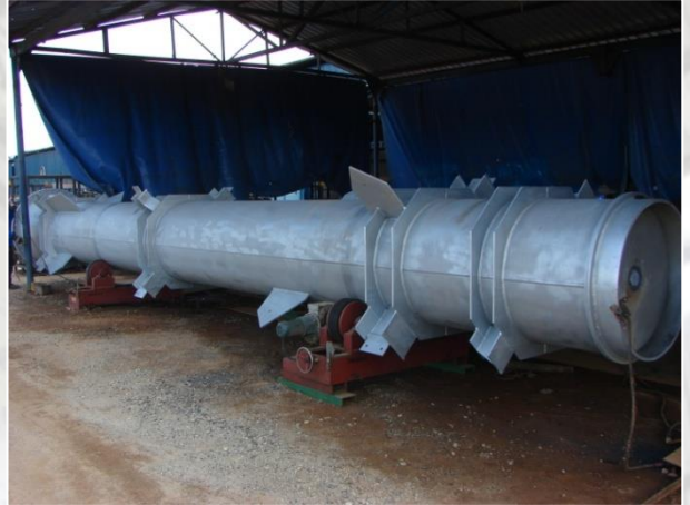
Galvanized Column [Carbon steel]
