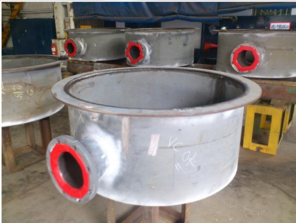
Roof Drain Sump [Carbon steel]
