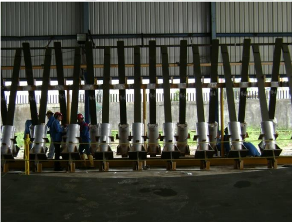
Anchor Strap [9% Nickel steel ,Stainless steel]
