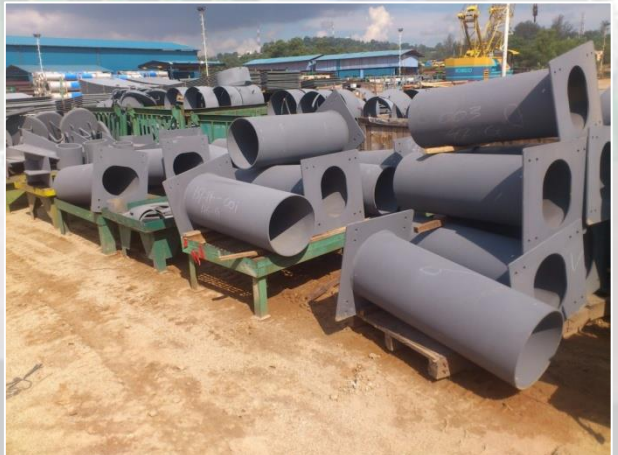
Guide Pipe [Carbon steel]
