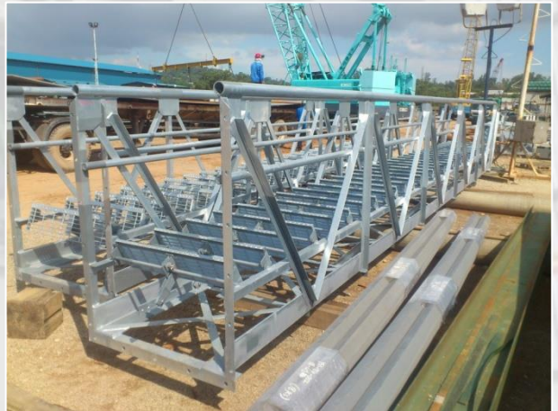
Galvanized Staircase [Carbon steel]
