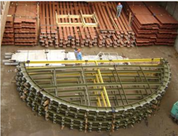
Center Ring for Dome Roof Tank [9% Nickel steel]
