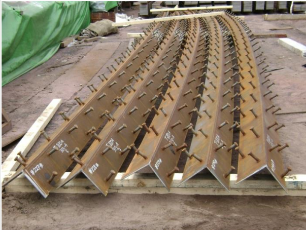
Corner Anchor with Stud Dubel [Carbon steel]
