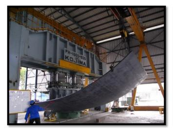
Batam Plant Equipment – 1,600 ton Press Machine
